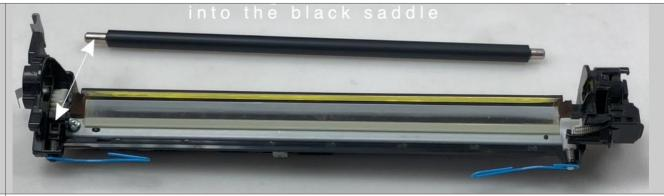
**30.** Reinstall the white part of the drive hub as shown
